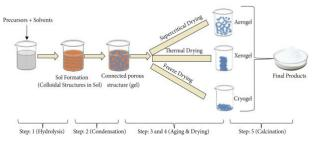
The solution is a suspension of particles in a liquid phase called a colloidal solution. The gel is an insoluble solid macromolecule. Due to itssimplicity and the ease with which the majority of nanoparticles may be created, solution gel is the most used bottom upapproach. It is a wet chemical method that uses a chemical solution as a precursor for an integrated system of discrete particles.
