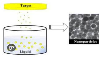
Sputtering is the deposition of nanoparticles on a surface by ejecting particles from it by interacting with ions. Sputtering typically involves depositing a thin coating of nanoparticles, followed by annealing. The substrate type, annealing temperature, and annealing time, among other factors [34].
