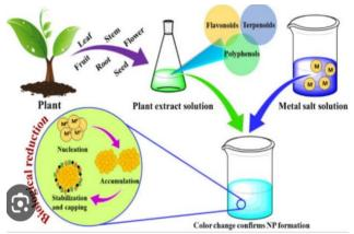
An ecofriendly method for creating non-toxic, biodegradable [28] nanoparticles is biosynthesised. Instead of using conventional chemicals, biosynthesis creates nanoparticles using precursors and elements like bacteria, plant extracts, fungi etc, and for bioreduction and capping applications. The biosynthesized nanoparticles have distinct and improved features that find use in biomedical applications [29].
