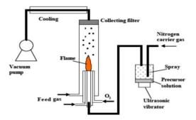
The most widely utilised method for producing nanoparticles on big scale is pyrolysis. It involves using flame to burn a precursor. The precursor is either a liquid or a vapour that is injected under high pressure through a small hole into the furnace, where it burns [26]. The nanoparticles are then recovered by air-classifying by product gases. Some furnaces create high temperature for simple evaporation by using laser and plasma rather than flame [27].
